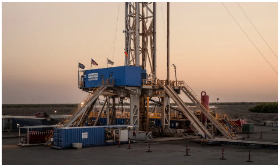
Sage Geosystems used a Nabors F-35 drilling rig at its geothermal test site in Starr County, Texas. It can drill to about 25,000 feet and lift and suspend 1 million pounds. PHOTOGRAPH : DAN WINTERS
